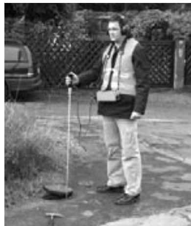
Picture 7: Points testing with listening rod at the W.A.S.
